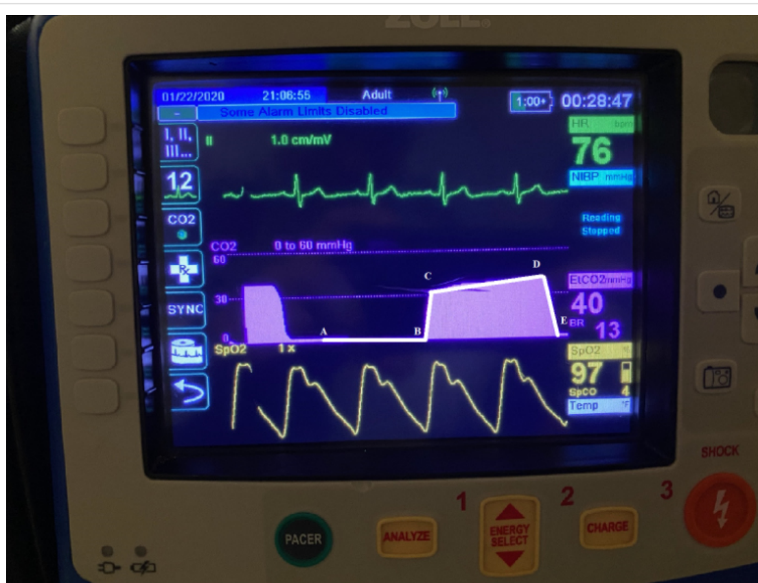
(Figure 1) A-B= Zeroed out baseline, B-C=Beginning of exhalation, C-D=Exhalation plateau, D=End-Tidal concentration that produces the numerical capnometry value, and D-E=Inspiration (Photo compliments to Dorchester County (SC) EMS for the use of their equipment.)
